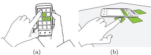
Fig. 3 Select&Place2Share allows users to select items that are intended for sharing (a). Then users place their phone on the surface and selected items are displayed around the phone (b).
